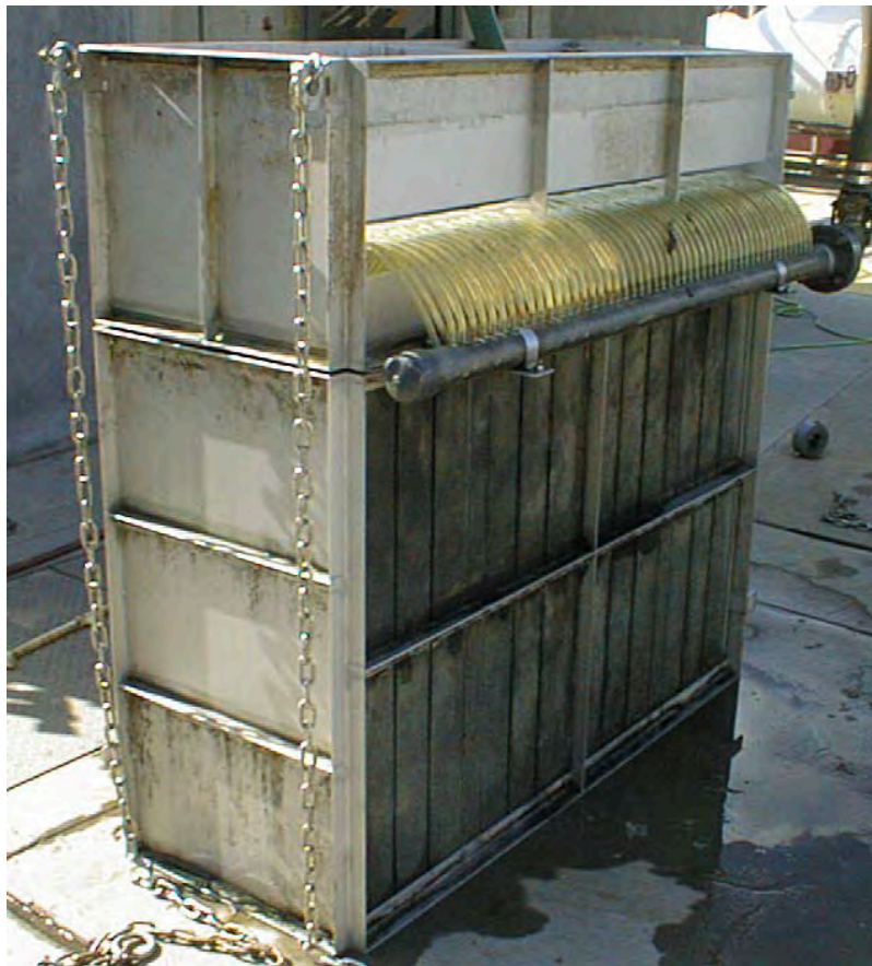
Kubota: Upper Membrane Cassette (top); Lower Membrane Cassette (bottom)
