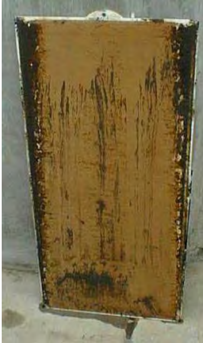
Kubota Type 510 Membrane (after 2 months operation)
