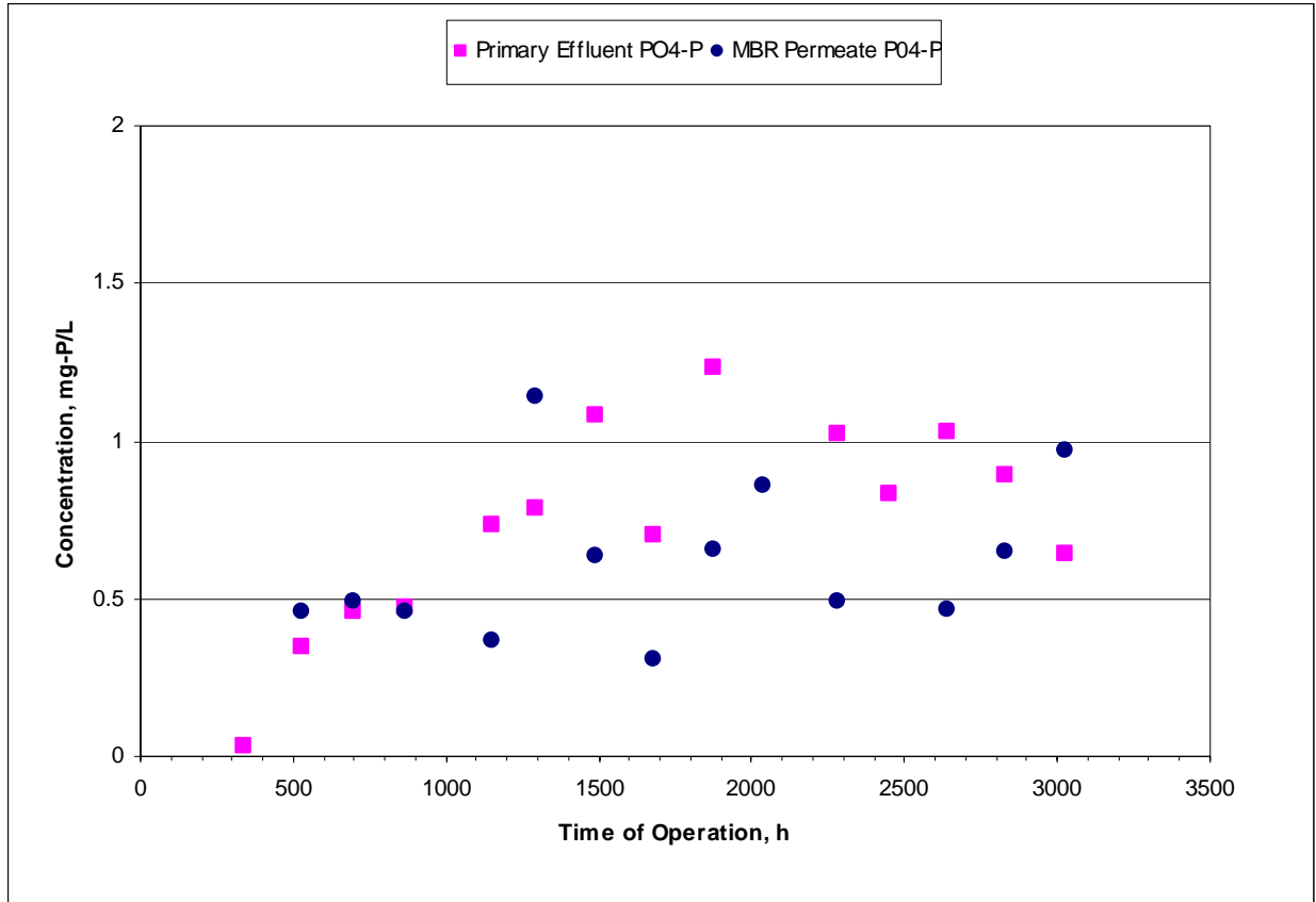
Figure 6-15: Ortho-Phosphate Removal by the Zenon MBR
